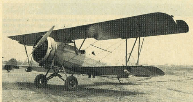
A Travel Air B-4000 with a Wright J-5 that was used by Parks Air College. NC475M was photographed at the Parks Airport about 1941. This was Parks' instrument trainer. Note the ailerons, landing lights and flare chutes. (J. Roby/AAHS)
