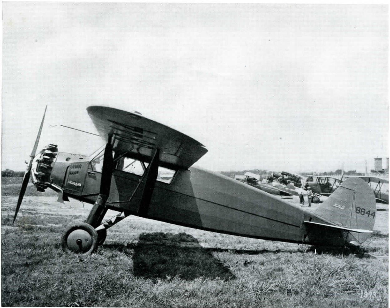
Side view of "Type 10-D" Cabin Monoplane
