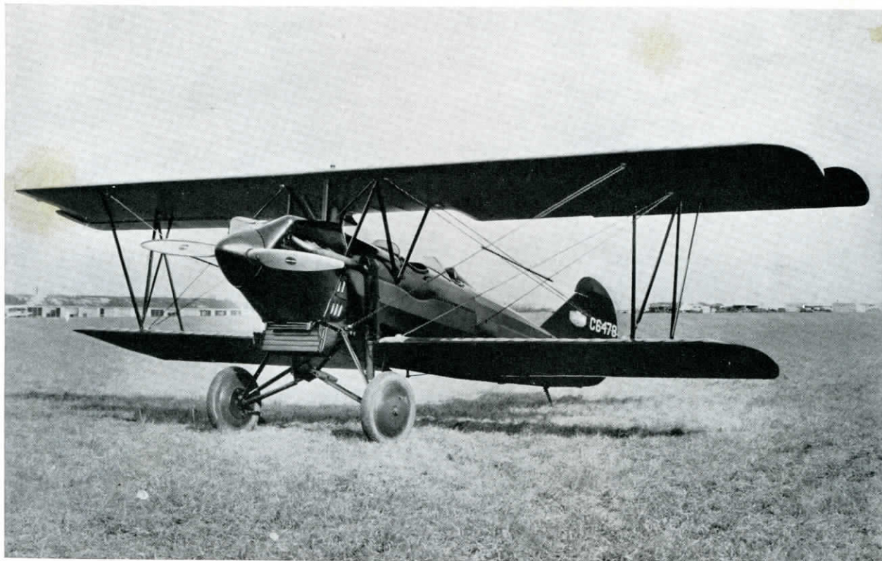
The Travel Air Type "3000" is the same type as the Type "4000" but with a 150 H.P. Hisso engine
